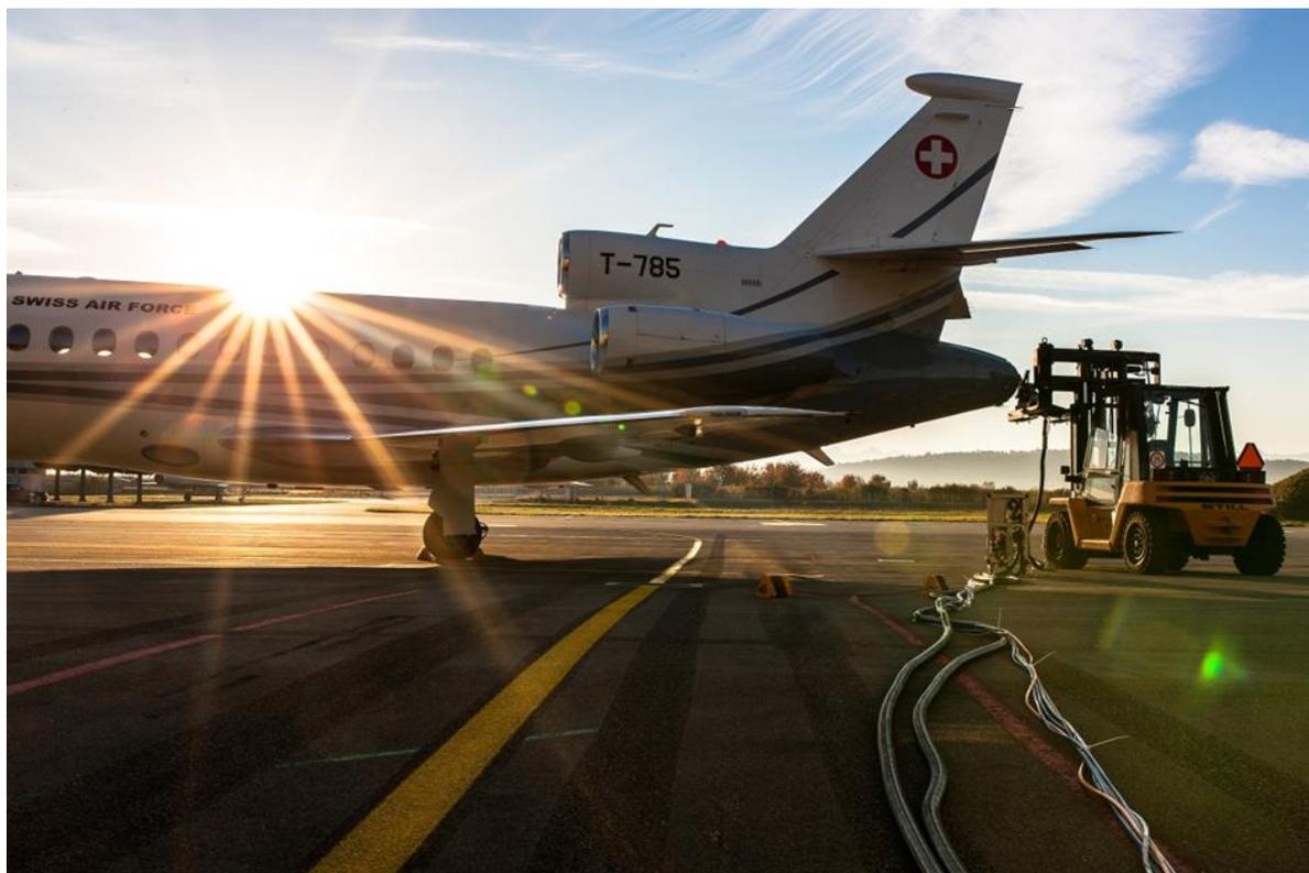
Sunrise above the Falcon 900 EX with the exhaust sampling probe and instruments in place. Photo: Lukas Durdina.
